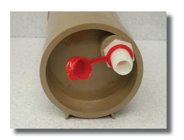
The photograph at the left shows the inflow side of the DD2011. Note that the inflow port is "off axis". This side of the separator is connected to the HVE line coming from the patient. Note the red vinyl cover over the 5/8 inch inflow port of the separator. When the separator is loaded with debris and needs changing, the red vinyl cover is placed over the port to prevent any leakage of debris from the separator.
