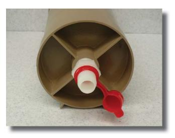
The photograph at the left shows the outflow side of the DD2011. Note that the outflow port is in line with the long axis of the separator. This side of the separator is connected to the vacuum source. Note the red vinyl cover over the 5/8 inch outflow port of the separator. When the separator is loaded with debris and needs changing, the red vinyl cover is placed over the port to prevent any leakage of debris from the separator.
